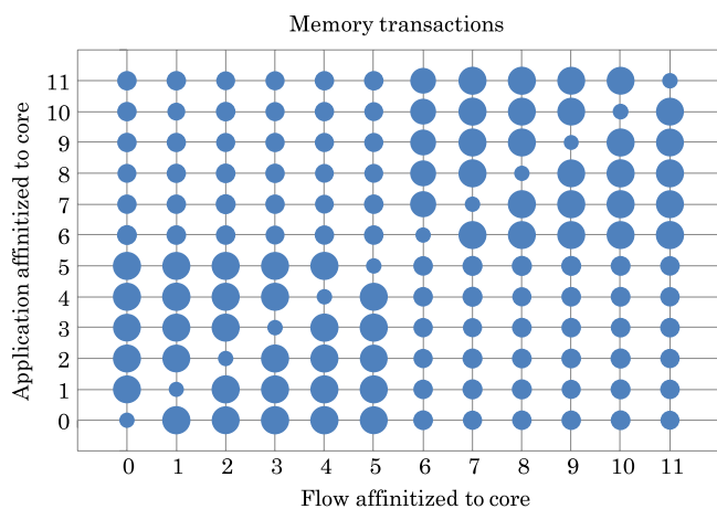
Fig. 6. The fraction of instructions retired/throughput dedicated to memory transactions (as measured by counter mem_trans_retired) for all 144 tests.
